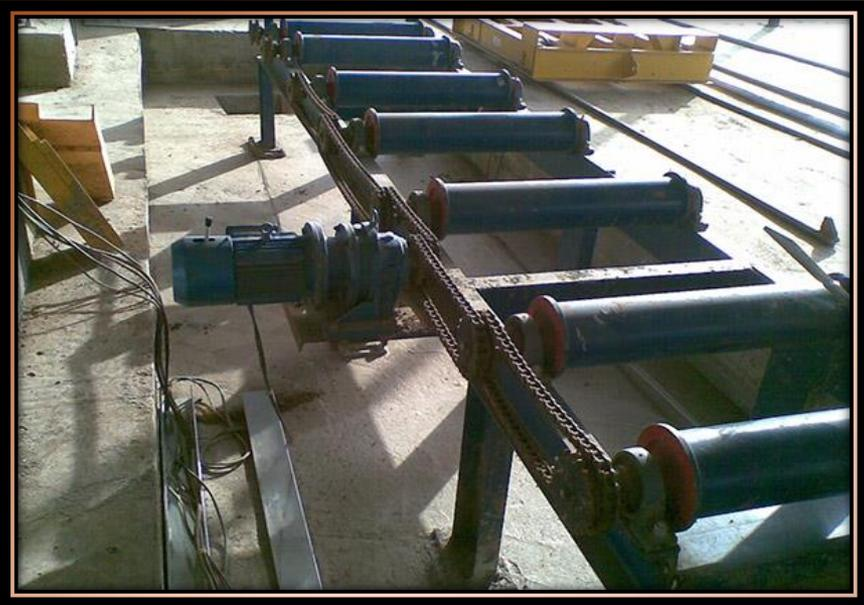
**Mould Roller Conveyors**
